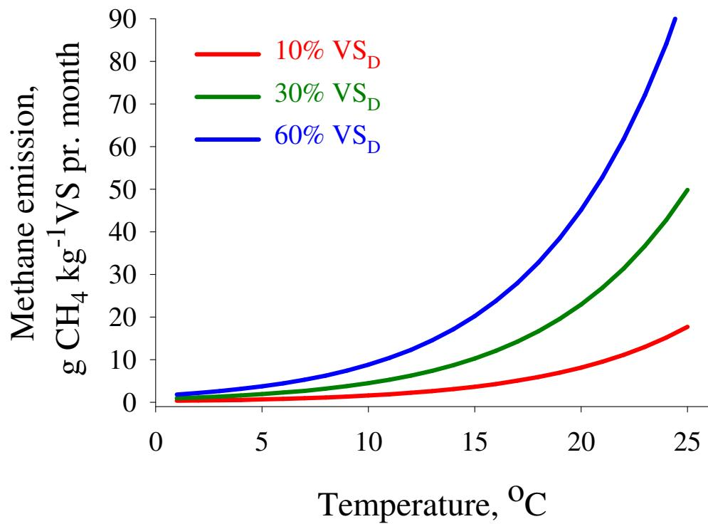
VS<sub>D</sub> is the fraction of manure that is digestible
