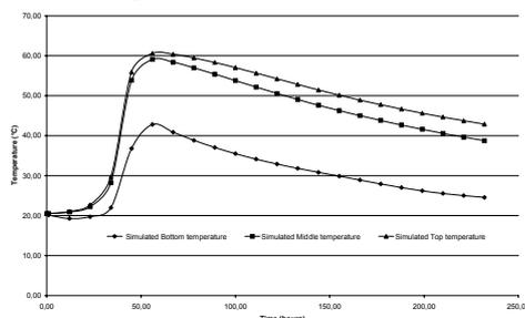
**Figure 1.** Temperature simulation within the composting pilot
