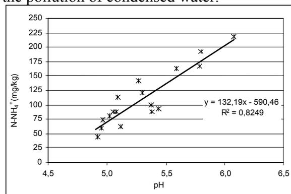
**Figure 2.** Correlation between free ammonia concentration as function of pH at acidification step
