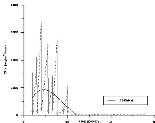
**Figure 2.** Gas emissions from windrow during composting process.
