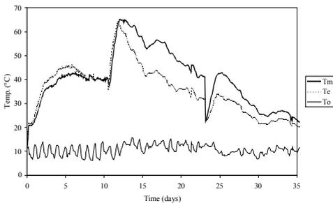
**Figure 1.** The average temperature at 10-minute intervals in the middle of the compost ( $T_m$ ), at one of the walls of the compost ( $T_e$ ) and in the surroundings ( $T_o$ ) for the pilot scale experiments.
