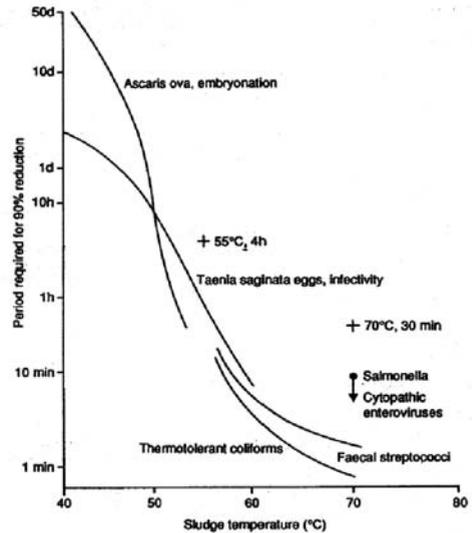
The two figures above express the effects of temperature and time on some species of microorganisms. In Figure 1 the *Safety Zone* is the area of the graph where pathogens would not survive, or the sludge would be virtually pathogen free due to a combination of time and temperature. Practical studies indicate that sludge should be held for four hours at 55°C (Fig. 2) or 30 minutes at 70°C to kill at least 99.99% of pathogens (Carrington et al., 1998).
