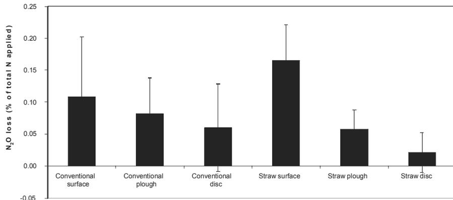
**Figure 3.** The influence of straw use and incorporation technique on total  $\text{N}_2\text{O}$  emissions (% of total N applied) following cattle FYM applications
