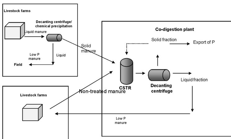
**Figure 2.** New concept for a co-digestion biogas plant integrating solid-liquid separation at selected farms.
