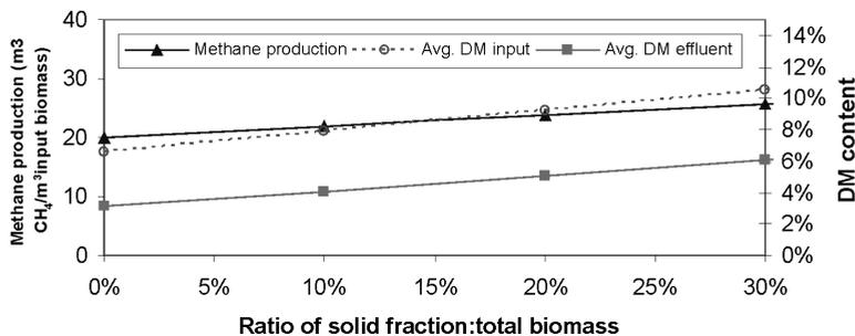
**Figure 3.** Methane production ( $\text{m}^3/\text{m}^3$  biomass input) and the average DM content in feed and effluent after substituting the existing biomass with increasing amounts of solid fractions from manure under the conditions listed in table 1.
