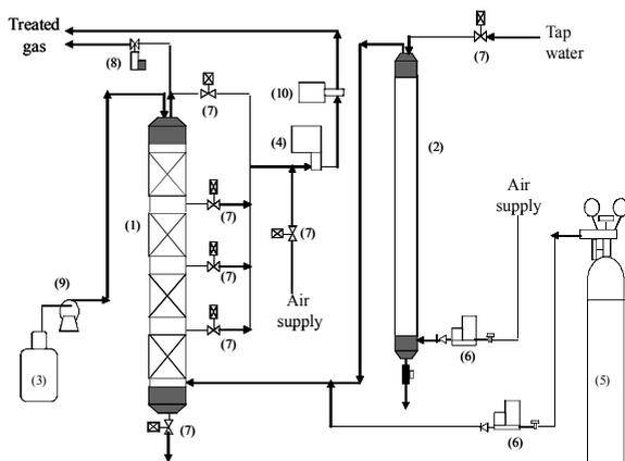
**Figure 1.** Schematic of the biofiltration pilot-plant. (1) Biofilter; (2) Humidification column; (3) Nutrients reservoir; (4) Relative humidity and temperature sensor; (5) Ammonia gas cylinder; (6) Mass flow controllers; (7) Normally closed electrovalve; (8) Normally opened electrovalve; (9) Pump; (10) Ammonia gas sensor.
