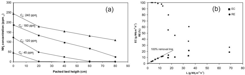
**Figure 2.** a) Ammonia concentration along the bed height; b) Elimination capacity and removal efficiency profiles for ammonia inlet concentrations of 45, 120 and 240 ppm<sub>v</sub>.
