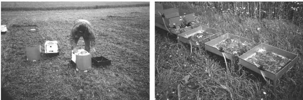
**Figure 1.** Equipment used for measuring a) ammonia emissions and b) leaching from cut plant material to soil.
