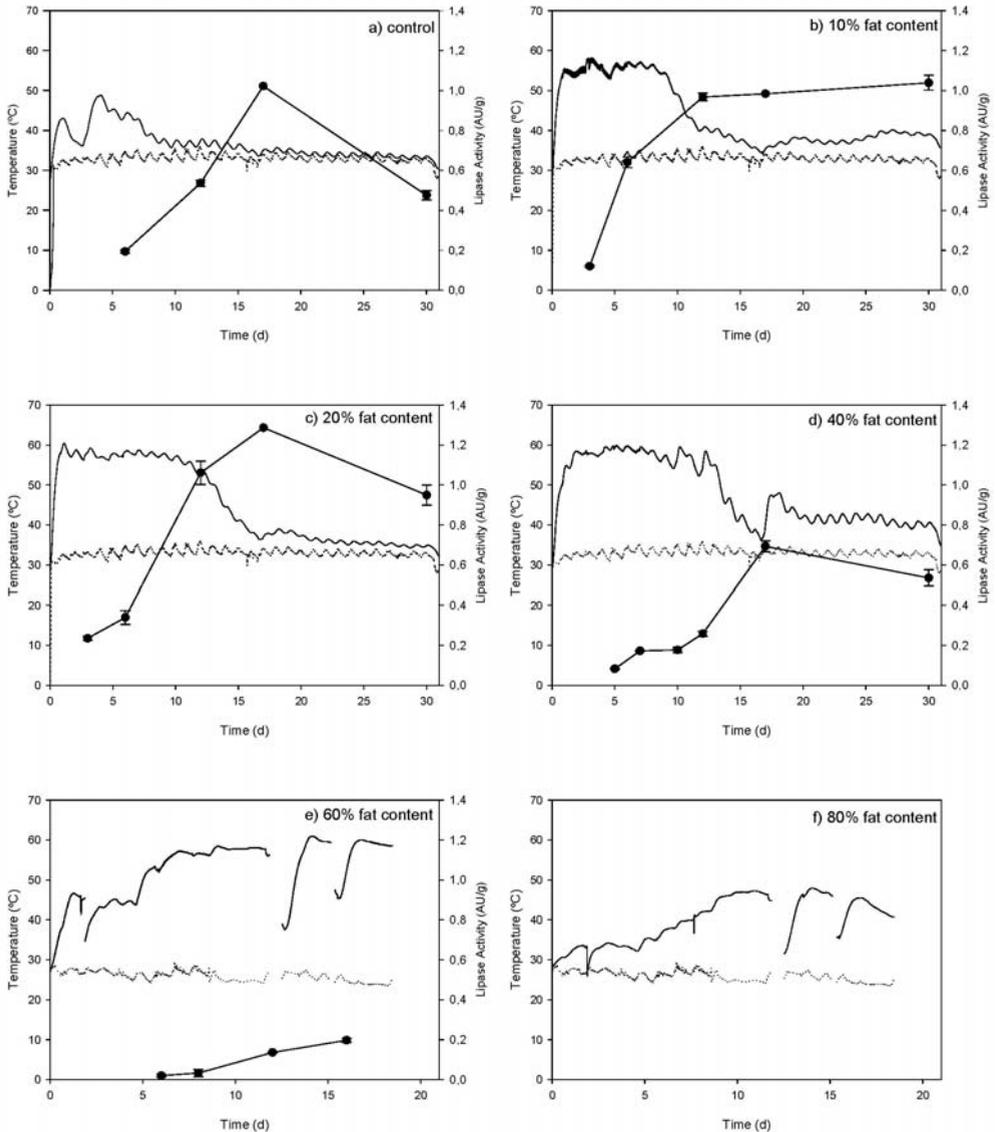
**Figure 1.** Temperature evolution (solid line), room temperature (dotted line) and lipolytic activity (circles) obtained in fat composting experiments.
