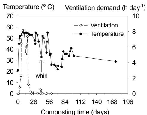
**Figure 1.** Evolution of temperature and ventilation demand during composting.
