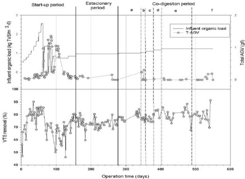
**Figure 1.** Performance of digester in set-up and co-digestion process
