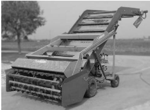
**Figure 1.** Composting equipment tested on separation of solids from swine manure.
