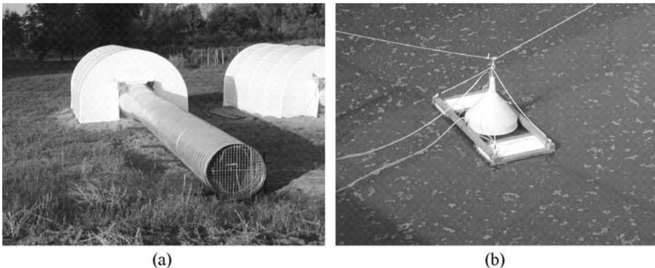
**Figure 1.** Devices used for ammonia emission measurement (a) Open Large Dynamic Chamber (b) the funnel system mounted on a floating device.
