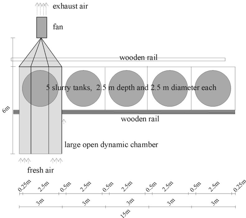
**Figure 1.** Design of the experimental facility for quantifying emissions from slurry stores (Amon et al. 2002).
